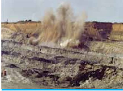
Deep hole heavy blasting operation
