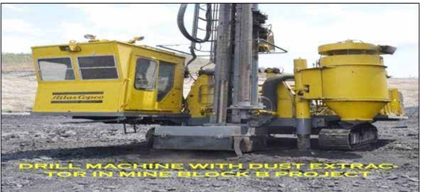
Fig. Drill Machine with dust extractors
