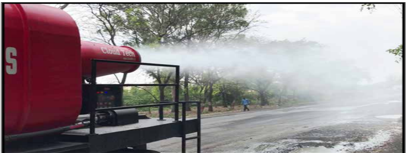
Fig. Fog canon for dust suppression at Nigahi OC of NCL
