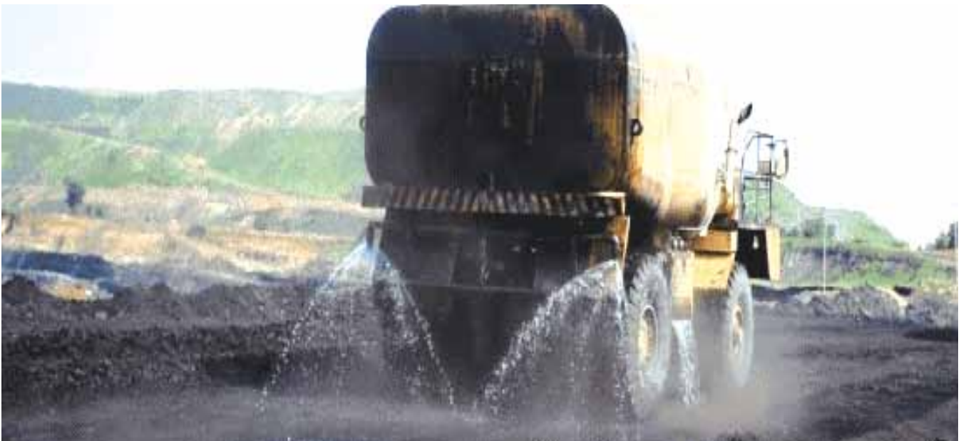
Fig. Mobile sprinklers in operation for suppression of dust
