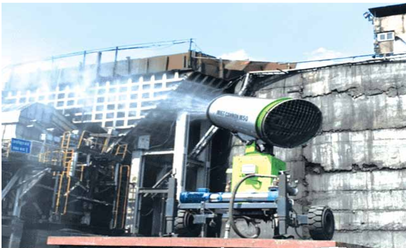
Fig. Mist Gun operation to control dust
