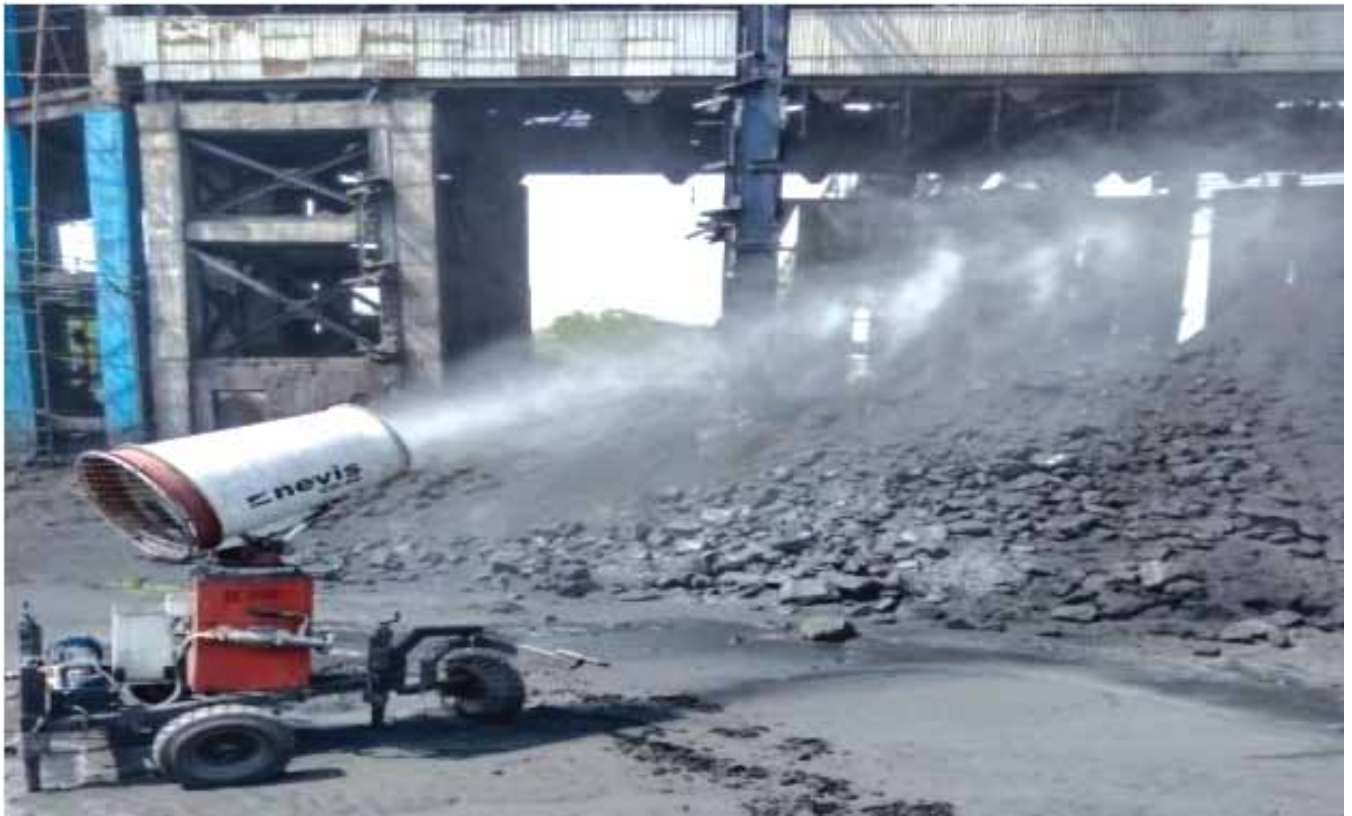
Fig. Fog canon working at RG OC-I CHP - SCCL
