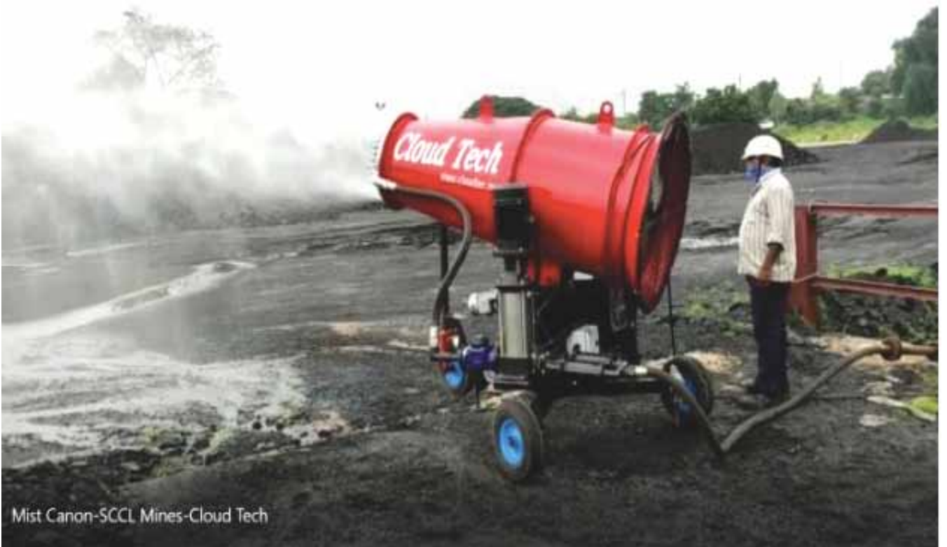
Fig. Fog cannon working at pit head CHP, JVR OC-SCCL
