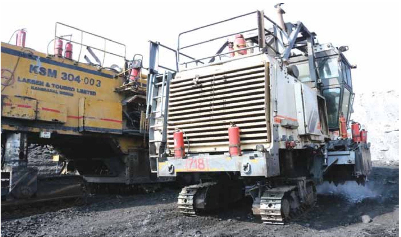
Fig. Surface Miner with water jets, Gevra OCP, SECL
