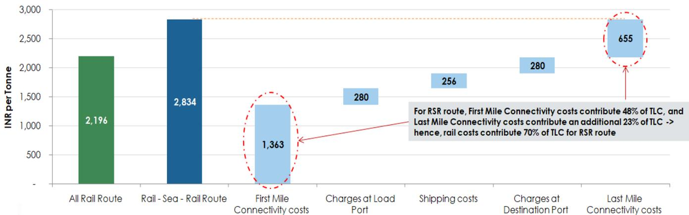
Thermal power stations in coastal areas of western states such as Gujarat and Maharashtra have existing coal linkages with SECL mines that are located at a significant distance from the nearest port. In this case study, we analyse the potential movement of thermal coal from SECL (Korba mines) via the All Rail Route and the Rail-Sea-Rail route (through Dhamra Port - as the Load Port, and Dahej Port - as the Destination Port).
