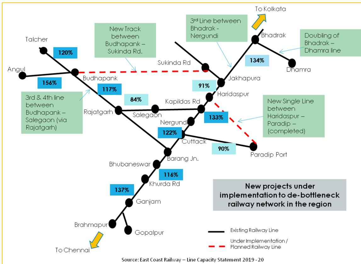
Several rail line capacity expansion projects for easing freight movement are under implementation and expected to drive traffic to ports (Paradip, Dhamra & Gopalpur) in the eastern cluster. Some significant port-rail connectivity projects such as the Haridaspur – Paradip Railway Line have been completed and operationalized (in 2021) and this is expected to improve rail connectivity to Paradip Port.
