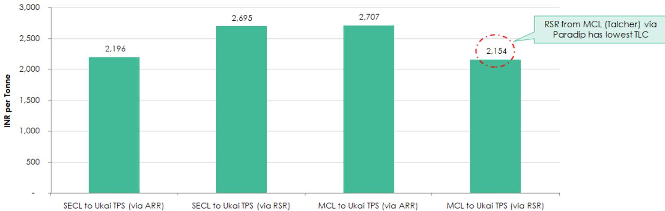
Thermal power plants located in Gujarat and Maharashtra have existing linkages with SECL, which is about 600 km from Paradip Port. Modification in the existing coal linkages from SECL mines to MCL mines can help reduce the first mile distance to around 200 km, and result in significant reduction in TLC.
