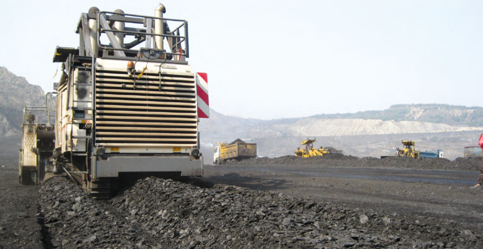
Eco-friendly 'Surface Miner' at Gevra area of South Eastern Coalfields Limited in Chhattisgarh
