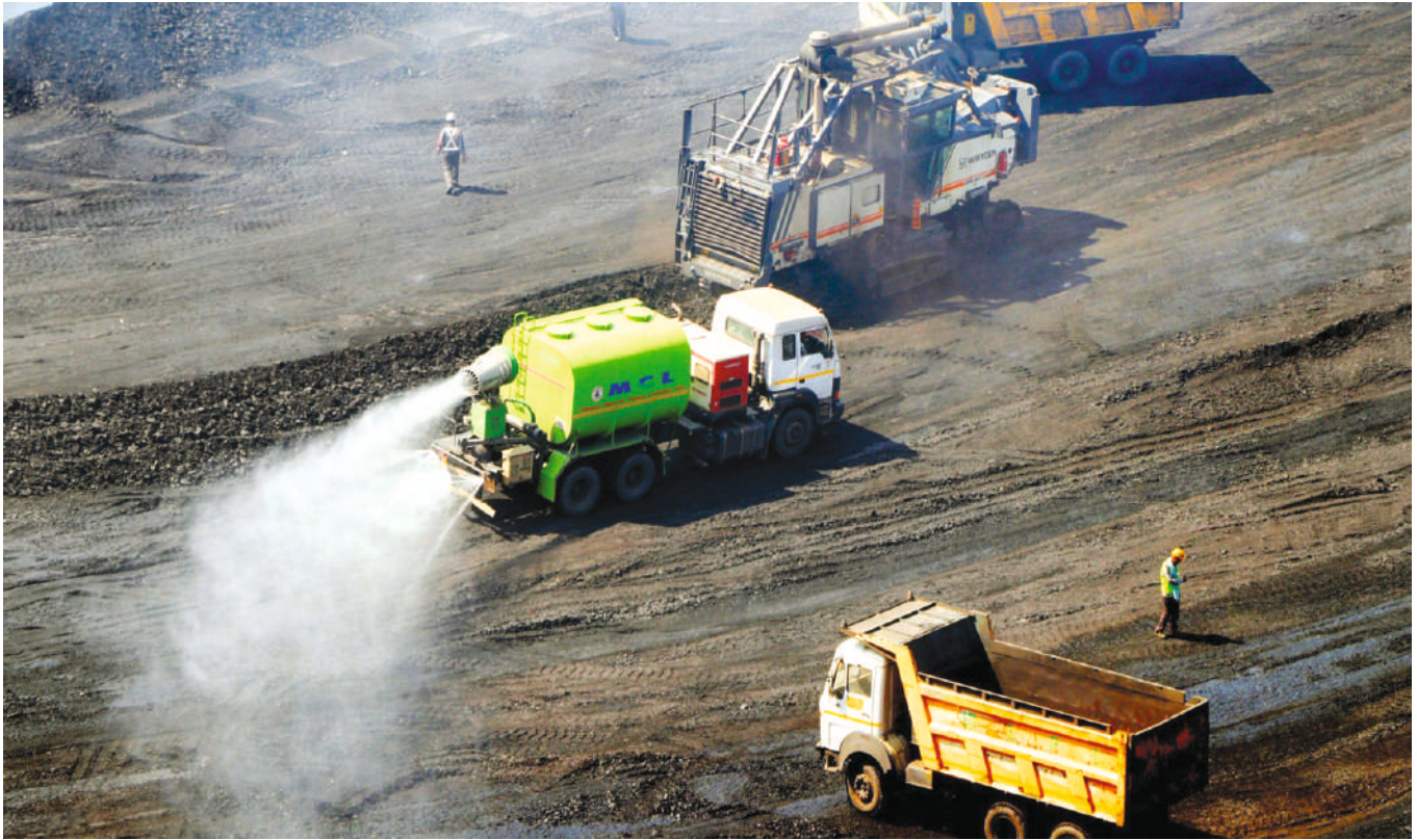
Fog cannon in action at Lakhanpur area of Mahanadi Coalfields Limited in Odisha
