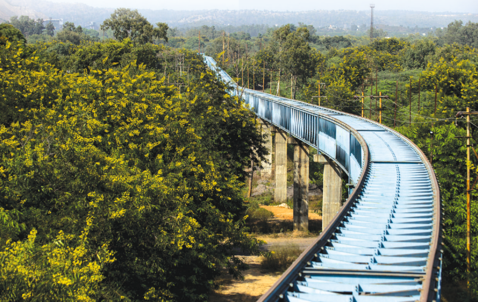
Coal transportation using eco-friendly belt pipe conveyor at Krishnashila area of Northern Coalfields Limited in U.P.
