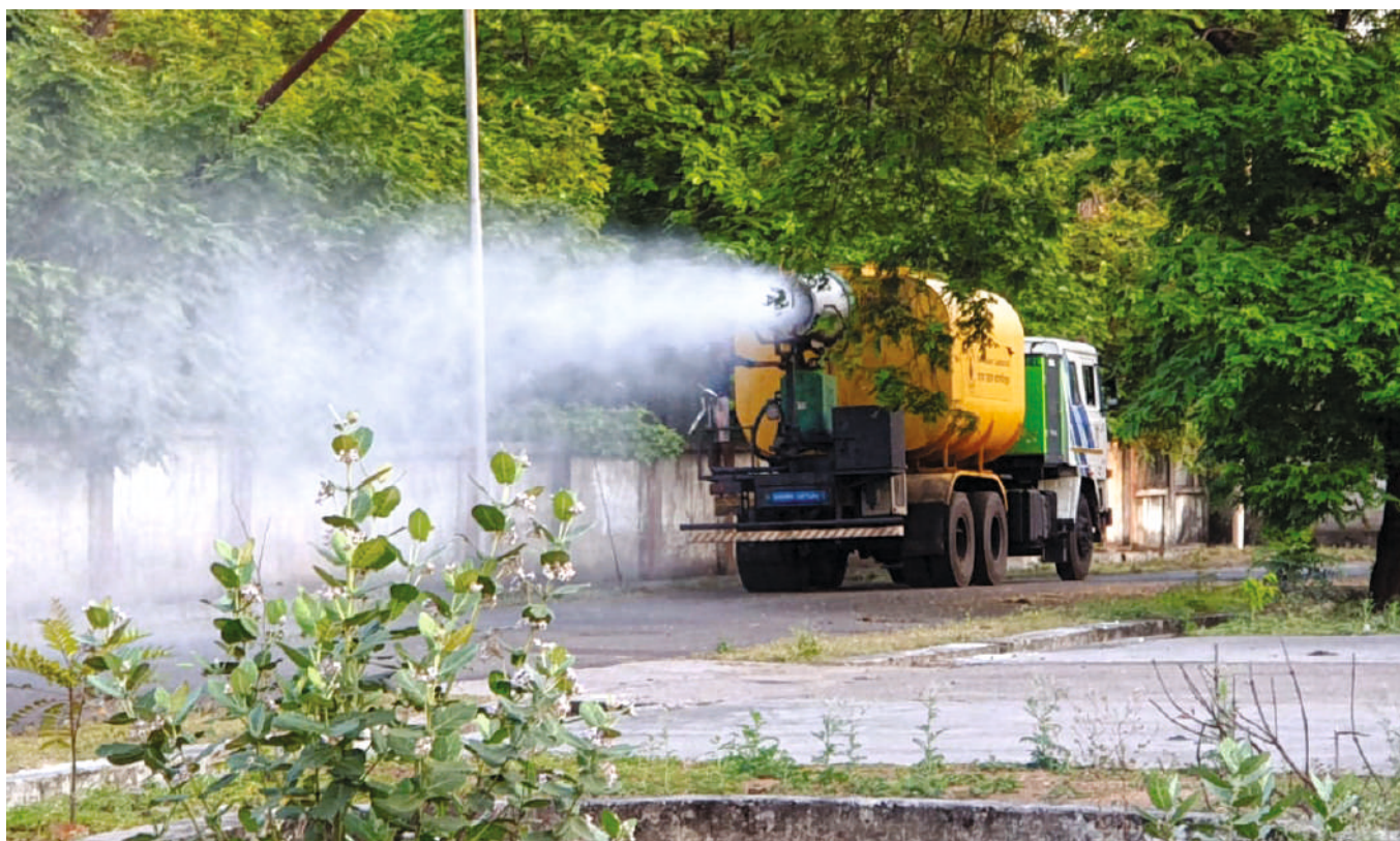
A fog cannon in action at Dipka area of South Eastern Coalfields Limited in Chhattisgarh
