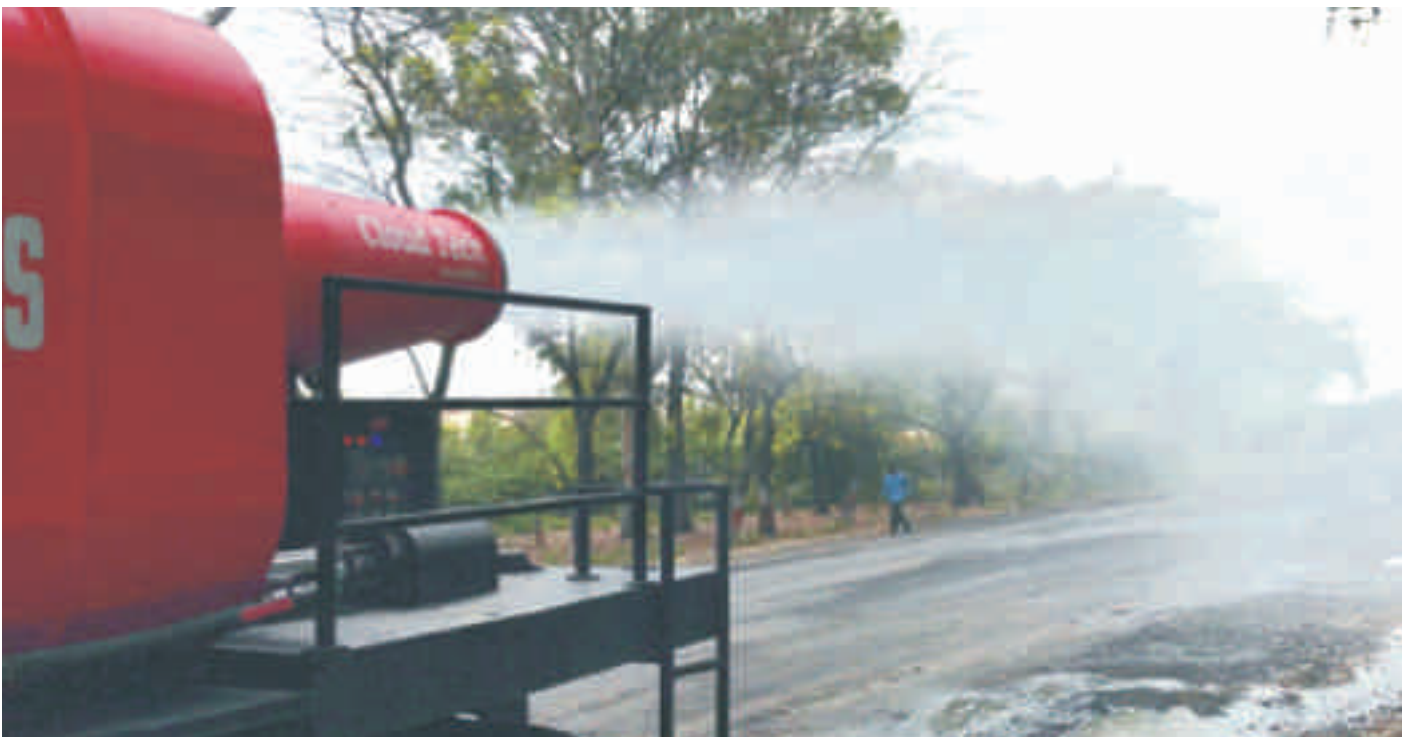
Fig. Fog canon for dust suppression at Nigahi OC of NCL
