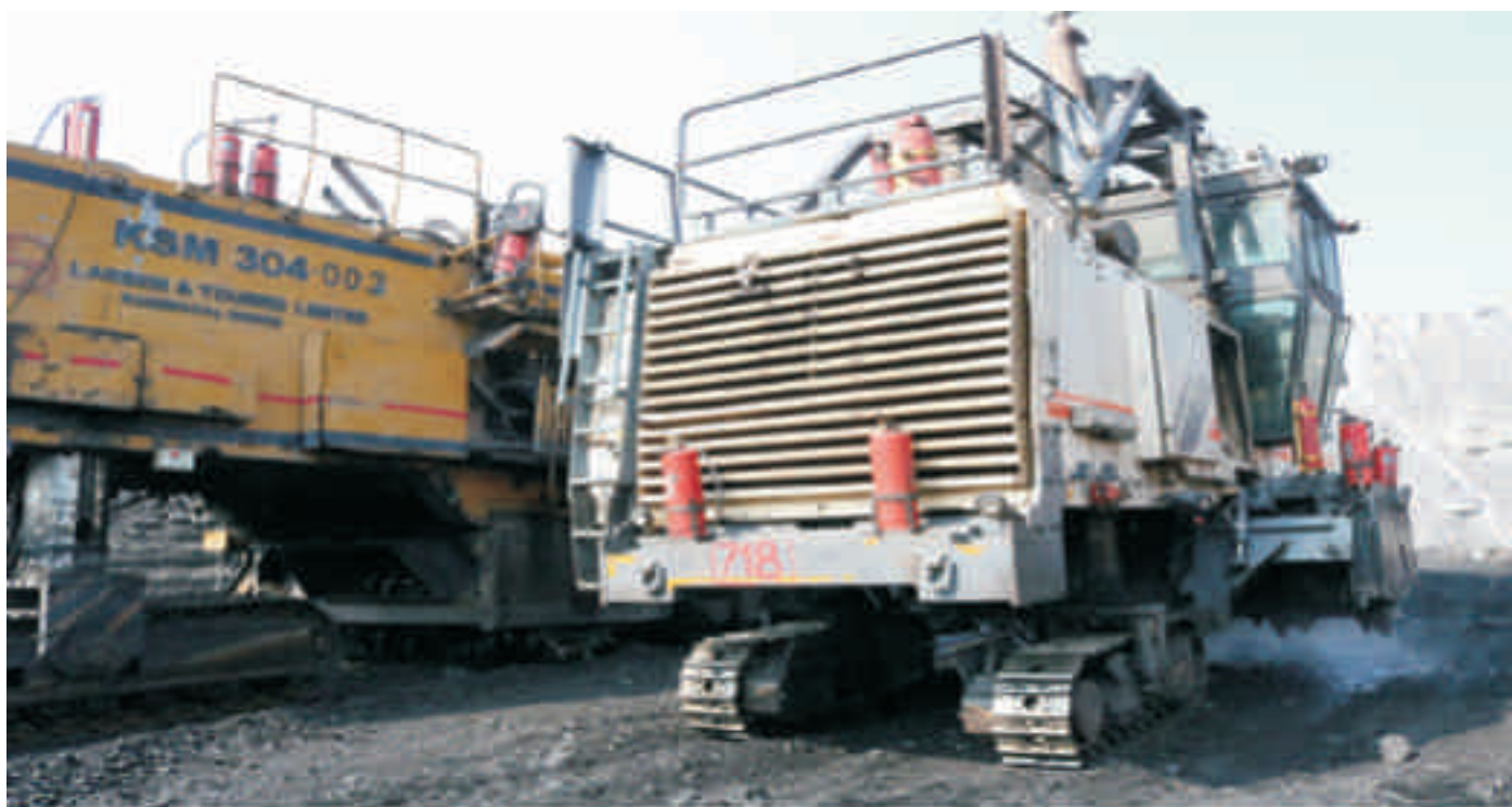
Fig. Surface Miner with water jets, Gevra OCP, SECL
