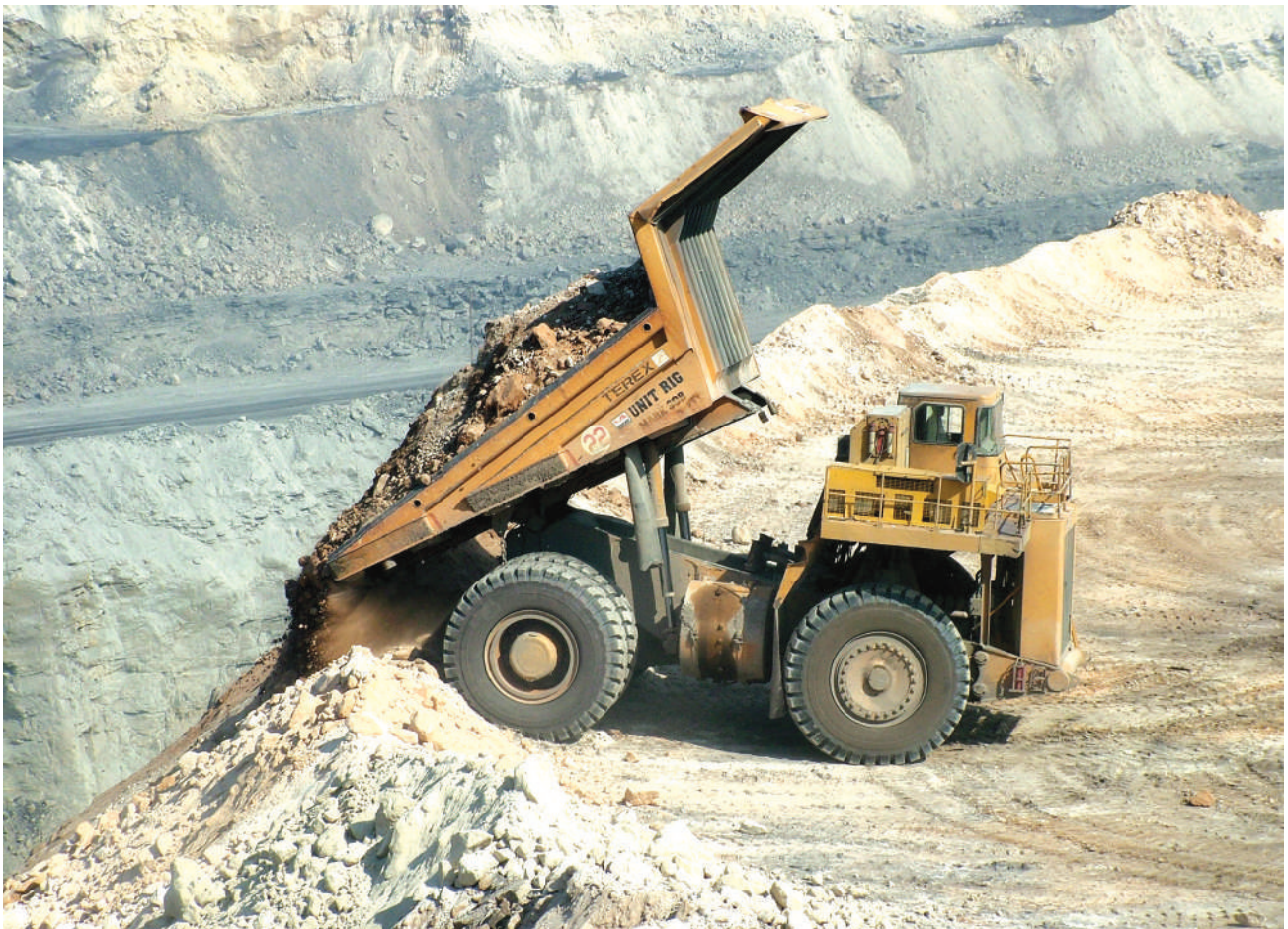
A heavy dumper unloading the overburden topsoil in opencast
