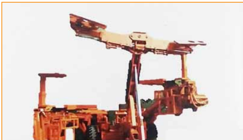
Roof Bolter-used for supporting the freshly cut coal roof by the continuous miner.
