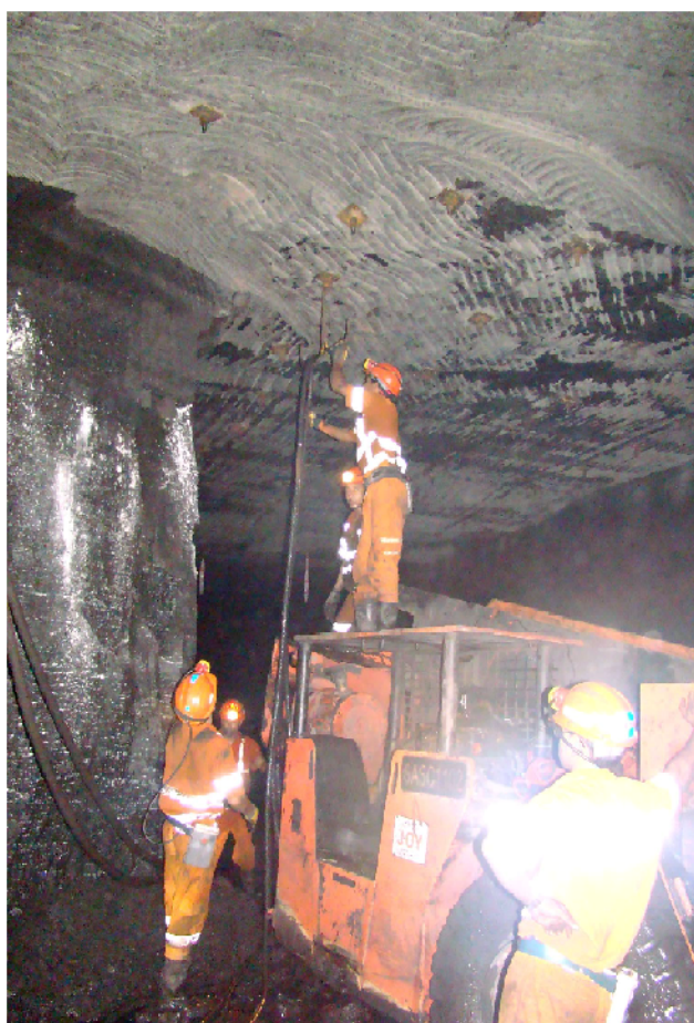
Mechanised Roof-Bolting process in progress for safety in an under ground coal mine
